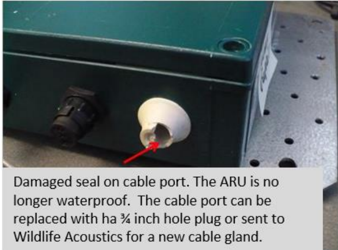
Figure 5: Example of a damage seal on the cable port.
