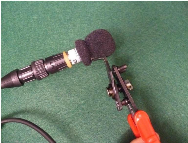
Figure 13: Using snap ring pliers to remove a microphone windscreen.
