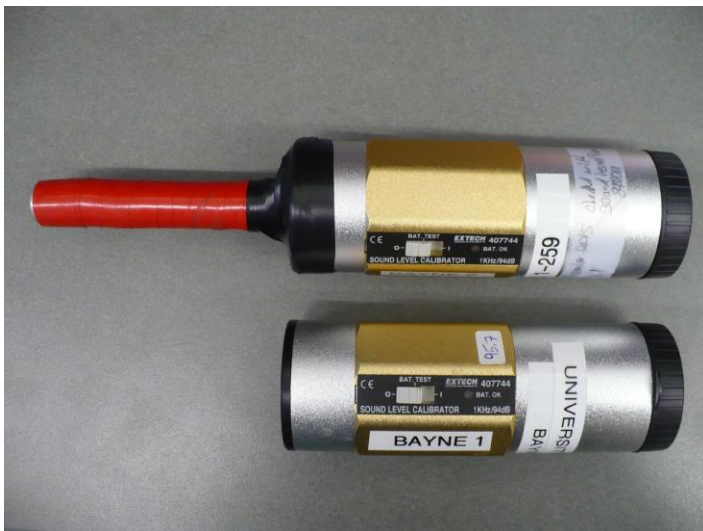
Figure 15: Extech calibrators. The upper one has a custom built adapter to reduce the test tone to 70 dB SPL.
