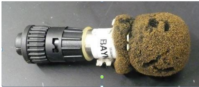
a. Damaged windscreen. Replace windscreen and test microphone.
