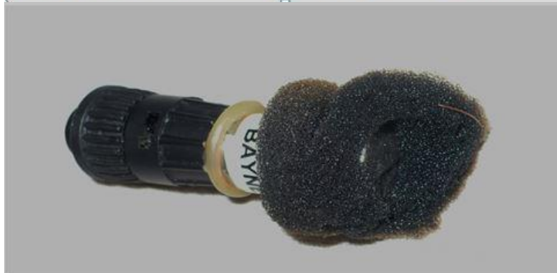
b. Damaged windscreen. Replace windscreen and test microphone.
