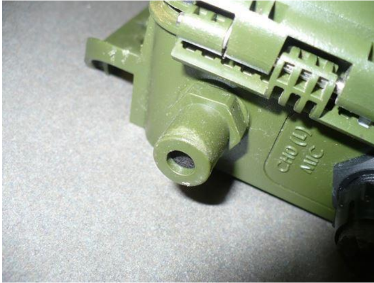
Figure 11. Damaged microphone: Test, if it records clearly, replace the membrane. If not, replace the microphone.
