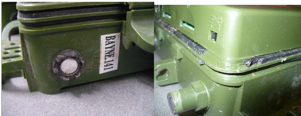
Figure 12. Left – Damaged vent: replace. Right – torn membrane: Small tears can be glued. If there are pieces missing, the seal needs to be replaced.
