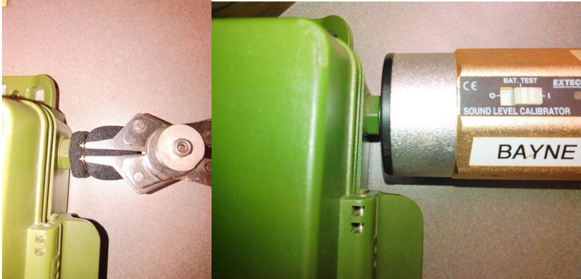
Figure 9: Right-Using snap ring pliers to remove a microphone windscreen. Left-using calibrator to test SM4 microphones.
