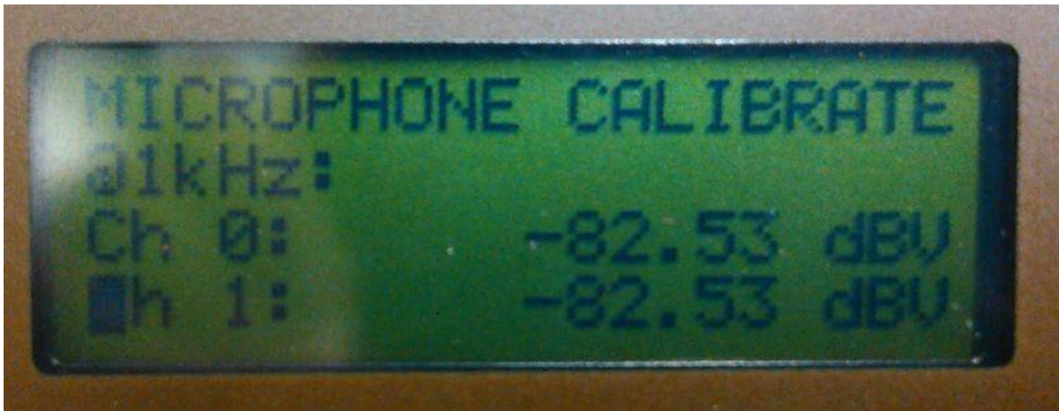
Figure 3: Calibration results showing balanced left and right channels. A 2 dB to 4 dB difference between channels is common due to the variation between microphones. Units need to be repaired if there are extreme differences between channels (>6 dB) or if one channel is not responding to sound.
