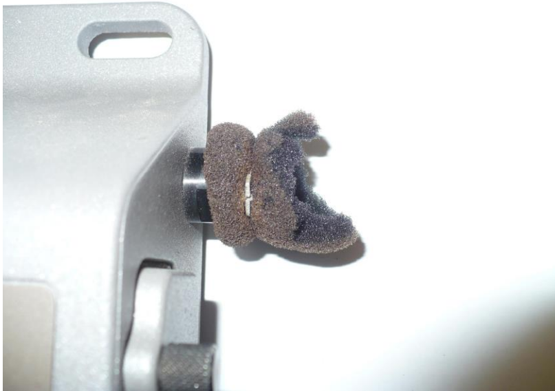
Figure 11: Damaged windscreen that needs to be replaced.
