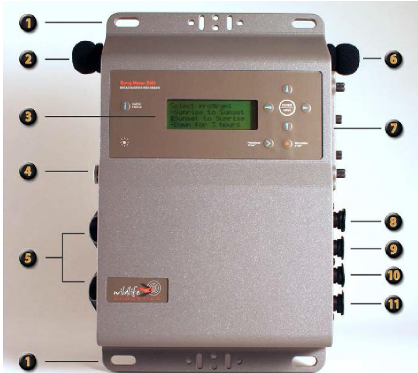
Figure 2: External image of an SM3 unit showing 1) built in brackets, 2 & 6) left and right microphones with windscreens, 3) LCD screen cover and keypad, 4) pressure vent, 5) battery bays, 7) metal cover and SD card slots, 8-11) external ports. (Image taken from Wildlife Acoustics SM3 User Manual)
