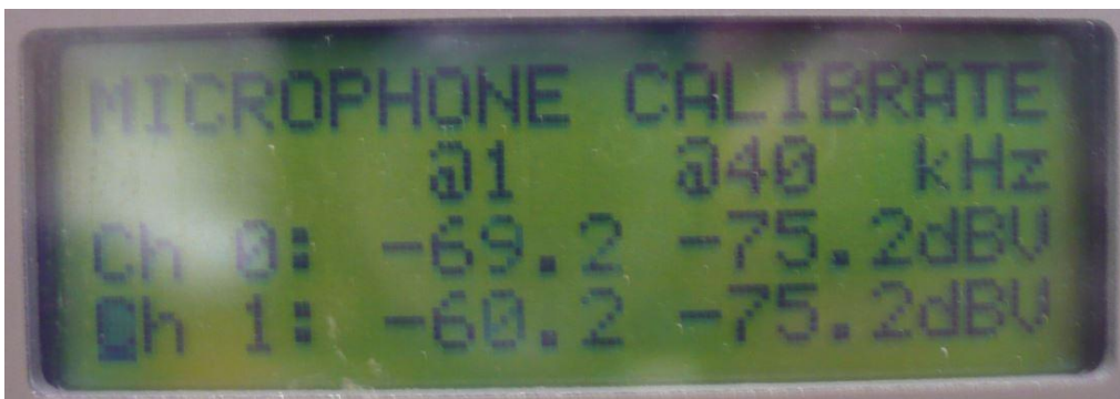
Figure 4: Calibration results showing unbalanced channels. A 2 dB to 4 dB difference between channels is common due to the variation between microphones. Units need to be repaired if there are extreme differences between channels (>6 dB) or if one channel is not responding to sound.
