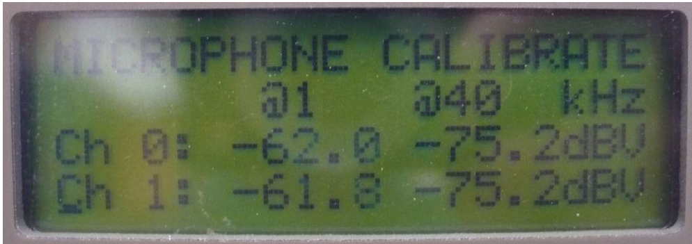
Figure 3: Calibration results showing balanced left and right channels.
