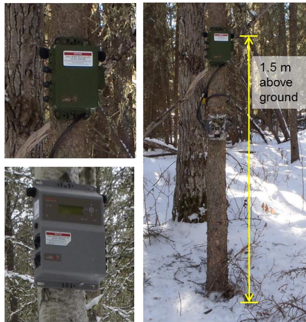
Figure 9. ARU placement on a tree. Microphones still are wider than the trunk, thus ensuring that sound is not blocked by the tree.
