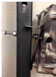
Figure 10. Custom A-bracket attached between the post and camera to adjust the tilt of the unit.
